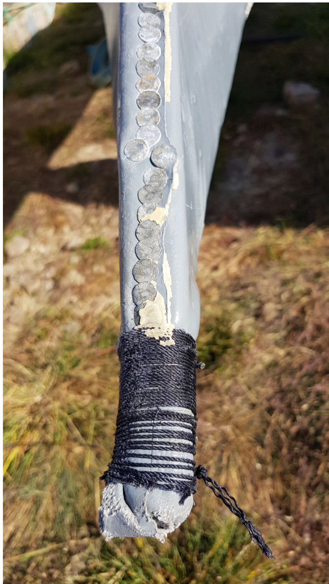
Whatever works: Roofing nails and twine keep this qajaq together.
