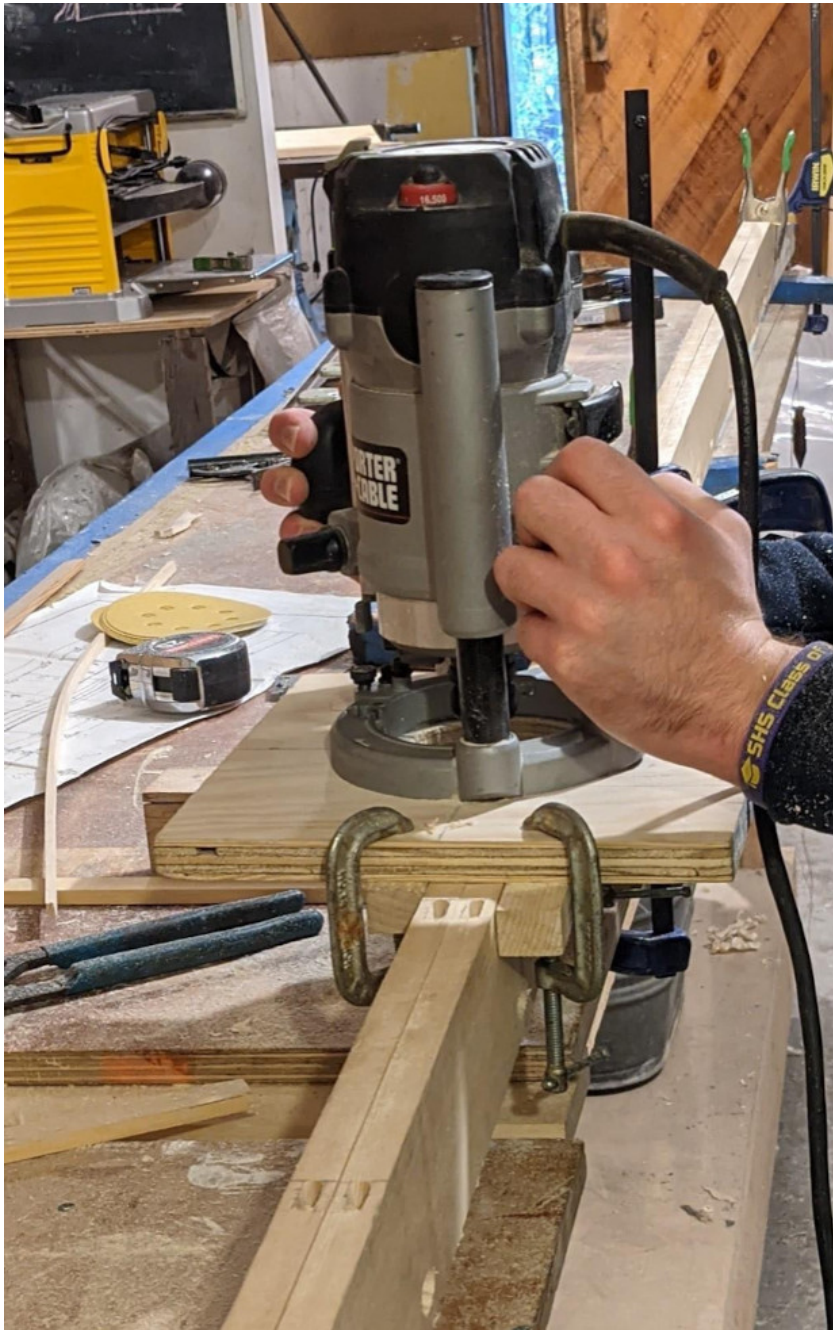
Above: router to cut mortises for ribs.
